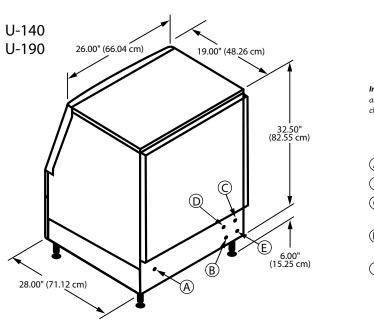
Installation Note Recommended clearance for top, sides, and back is 5" (12.7 cm) however, there is no minimum clearance required.
